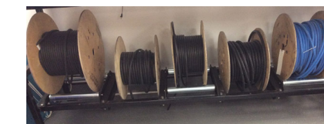
Cable drum storage on rollers
