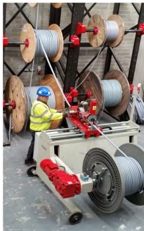
Jones Engineering Electrical Department cutting cable to length in Kildare facility for projects all over the country
