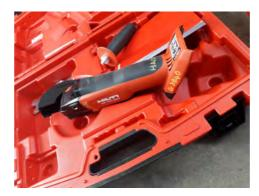
These tools are supplied with handles so as to keep control of the tool. They are not meant to be used with one hand. The majority of accidents with drills and grinders are because the user didn't have the handle fitted and therefore had no control of the tool when it got stuck or jerked. Workers have been thrown from ladders when a drill bit got stuck after hitting steel whilst drilling into concrete ceilings.
