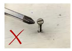
You'd be a long time trying to drive this screw in with the screwdriver shown and you wouldn't use a small screw gun (below) to drive a big masonry bit.
